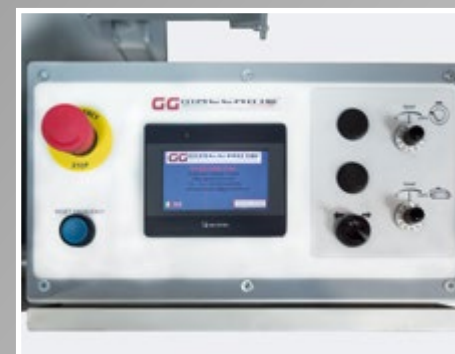
The functions are managed from the control panel with a colour touch screen, connected directly to the PLC control, which manages all functions of the machine. The ability to store a list of recipes allows custom programming according to the packaging requirements of each product.
