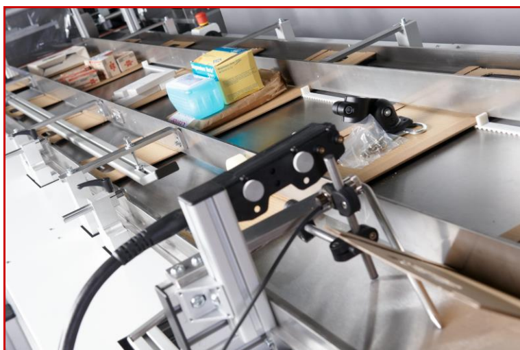
Automatic folding of the box and printing of the barcode with an ink jet printer
