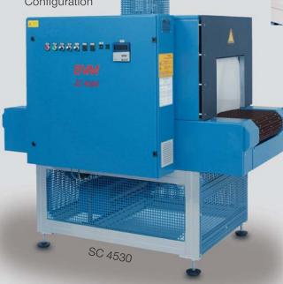
Air flow inside the insulated heat chamber is finely controlled by four dampers - top and bottom on two sides; the dampers are independently adjustable from outside the tunnel.
