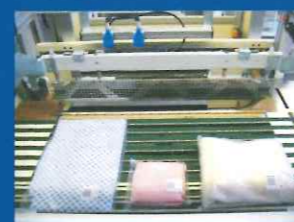
Capacity increase on the side sealing station with production capacities up to 1800 products per hour (patent-registered).
